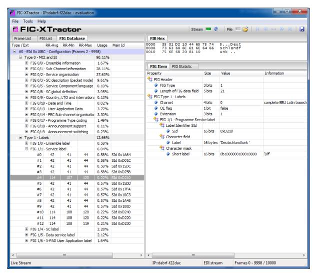
Figure 20 – The FIC-XTractor window with its three views to the FIC content
