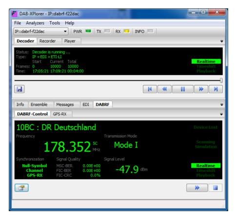
Figure 12 - Main window with Decoder and DABRF panel
