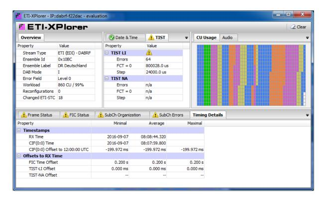
Figure 18 – ETI-XPlorer window with timing information from DABRF
