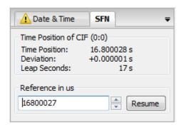
Figure 17 – Panel in ETI-XPlorer window showing the temporal position of the received RF signal of UEB400DXP
