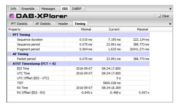
Figure 21 – New functions for EDI analysis coming with DABXP-OPL in the main window
